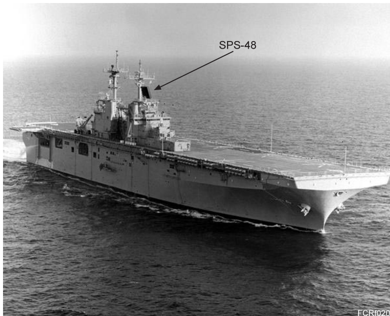
Figure 2-2.—SPS-48 series radar on USS Boxer , a WASP class amphibious assault ship.
